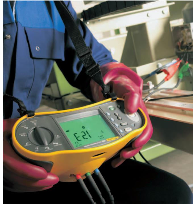
The Fluke 1650 Series Multifunction Installation Testers combine voltage, frequency, polarity, and short-circuit functions, along with multiple resistance functions and several functions for testing RCD's (residual current devices). The Fluke 1653, shown here, adds an earth resistance function, phase sequence indicator, and an IR port for uploading of measurement data to a computer.
