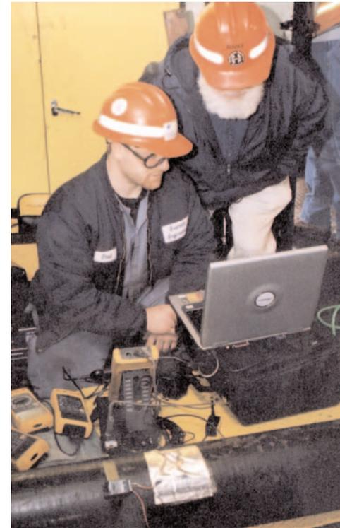
Paul Visocky of Everett Engineering and Chuck Newcombe of Fluke. Downloading data from three Fluke 189 DMMs and a Fluke 123 ScopeMeter into the laptop for comparison and analysis in FlukeView® Forms.
