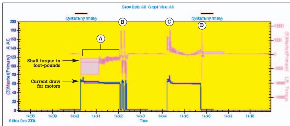
Figure 2. A—marks where the bridge began to raise. B—marks where the bridge is completely open and shaking. Note how the shakes cause the motor to turn on and off, as evidenced by the current draw. C—marks where the bridge begins to close. D—marks where it is settling into place.
