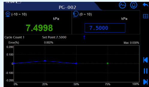
Pressure gauge / transmitter / switch calibration
